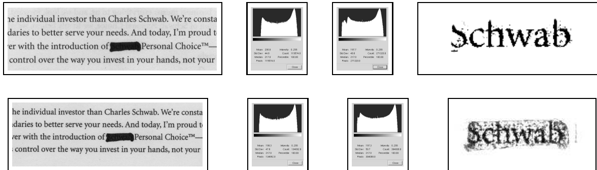
Figure 2: A portion of a redacted page. The top row represents scanned images of the redacted original. The bottom row represents a photocopy. From left to right we have the source image, the histogram of the “background” consisting of portions of the image not including the redacted word, the histogram of the entire redacted image showing the extension of the dark portion of the histogram, and the redacted region after the histogram analysis yields threshold values.
