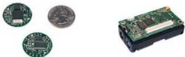
(a) MICADOT mote (b) MICA2 mote without sensor board
