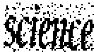
Figure 4. Example of a PessimialPrint challenge: an English word is chosen at random, then the word (as a whole) is typeset using a randomly chosen typeface, and finally the word-image is degraded according to randomly selected parameters (within certain ranges) of the image degradation model. Judicious choice of image restoration preprocessing can make character-segmentation straightforward.
