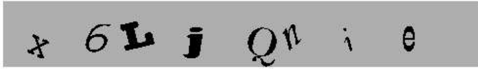
Figure 1. Example of an AltaVista challenge: characters are chosen at random, then each is assigned to a typeface at random, then each character is rotated and scaled, and finally (optionally, not shown here) background clutter is added. The fact that the characters are spaced widely apart invites segment-then-recognize attacks.
