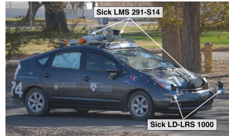
Fig. 1. The toolbox is branched from the source code used by the Ben Franklin Racing Team during the DARPA Urban Challenge. Our entry – Little Ben – employed five Sick LMS 291 and LD-LRS LIDARs during the race and was one of only six vehicles to successfully complete the 55 mile Urban Challenge Final Event. Ben ran on fewer than 5,000 lines of Matlab script – using mex interfaces to device drivers and messaging.
